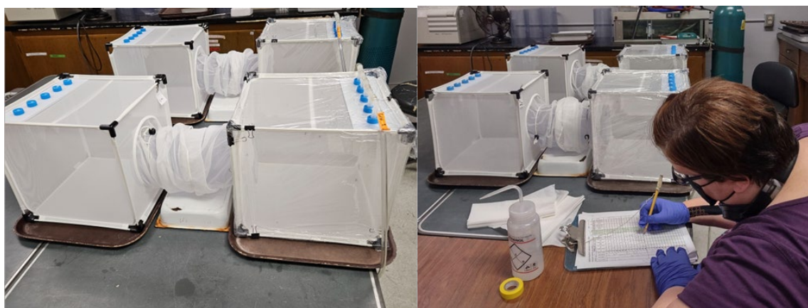
Figure 1. Assay chamber for repellent testing: Left image - Adult mosquitoes moved freely between repellent (right) and escape (left) cages via a connected PVC pipe. Right image - A spatial repellency trial being conducted in the laboratory.
