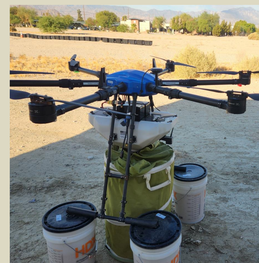
Drone shown above is calibrated with spinner on Drone illustrated above is Leading Edge's Precision Vision 35 X
