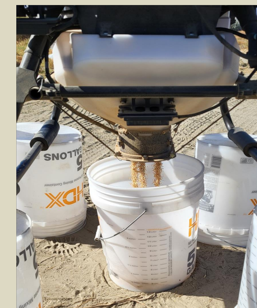
Drone is calibrated with spinner off, product collection shows little impact with spinner off. (Hyllo AG-230)
