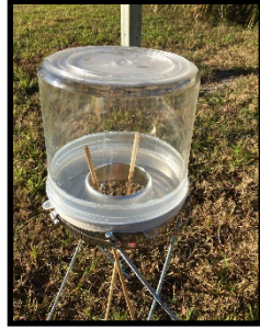
Fig. 3. Redesigned fire ant alate trap with dowel rods that guide alates into a collecting pan. Alates typically crawl to a high perch when they initiate mating flights.
