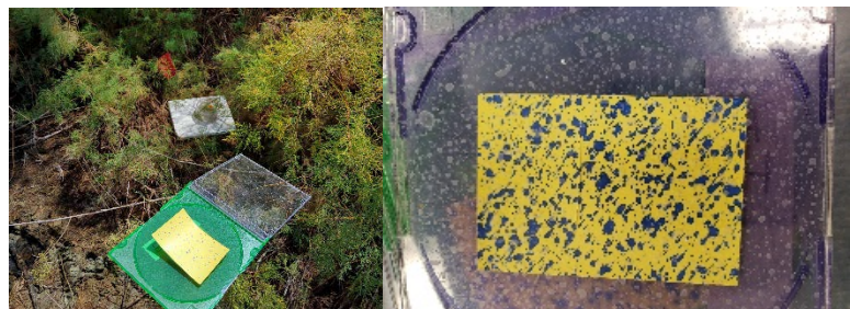
Left: Evaluation site with a card in the foreground and a cup in the background. Right: Card after application; the blue dots indicate droplets landed.
